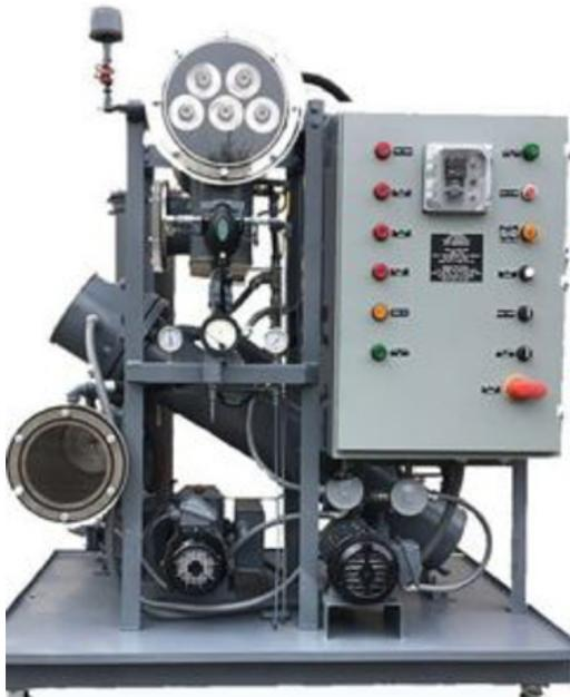
Figure 1. RIG Vacuum Dehydration Oil Purification Unit
