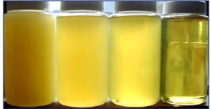
Figure 2. Example of oil with emulsified water content and oil after moisture removal is complete.
