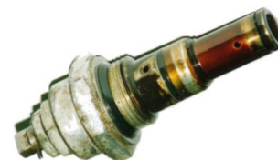
Copper colored varnish forms on lubricated components when oil becomes oxidized.
